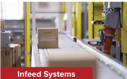
QSP models typically feature zero-pressure, 24-volt conveyors specified for their performance, safety and energy-efficiency.
