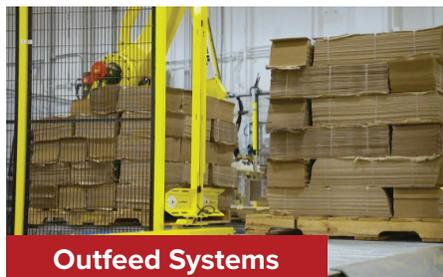
Pre-engineered pallet stations can be designed for manual operation or feature integrated discharge conveyors for a higher level of automation.
