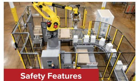
All cells are designed and configured with the appropriate safety fencing, light curtains and other systems to comply with category 3 safety standards.
