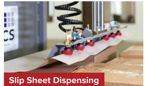
Quick-Ship Palletizers can be designed with a slip sheet hopper and standard EOAT that automates the placement of anti-slip sheets on each pallet.
