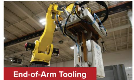
Multiple pre-engineered, in-stock EOAT units are available including our popular clamping tool with pneumatically-powered support lip.
